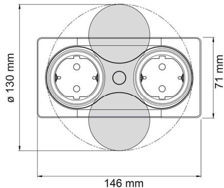
Mounting on horizontal or vertical panels of **5 to 40 mm**
