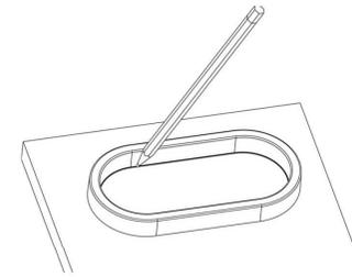
Easy cutting of the 135 x 60 mm hole thanks to the **included template**
